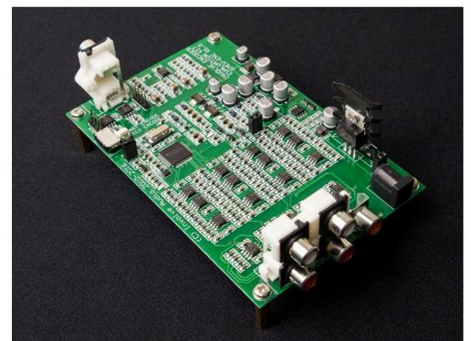
Both the Encoder and Decoder evaluation boards require 9V 1.66a power supplies – you can supply this yourself into the 2.1mm DC jack, or a suitable power supply can be provided for an additional USD \$10.
