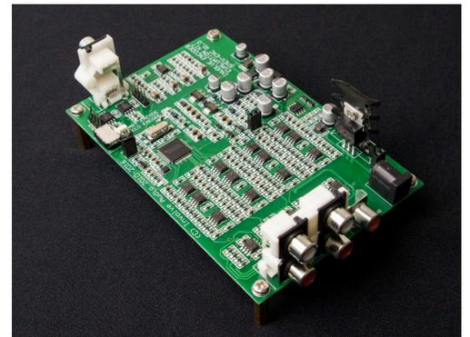
Both the Encoder and Decoder evaluation boards require 9V 1.66a power supplies – you can supply this yourself into the 2.1mm DC jack, or a suitable power supply can be provided for an additional USD \$10.
